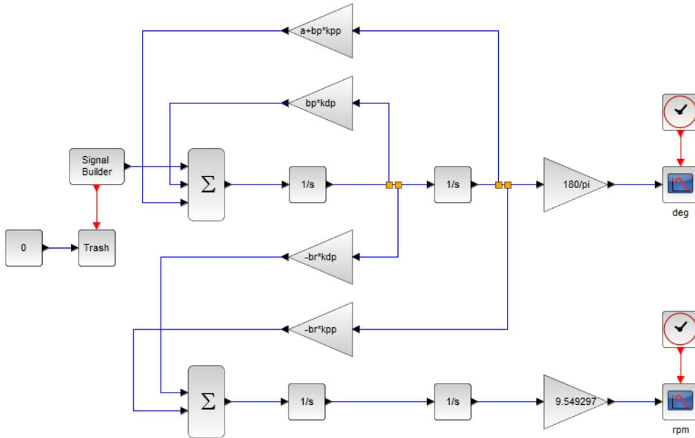
Fig. 2. Subsystem for working out a solution to system ODEs (4) (pendulum angle)
