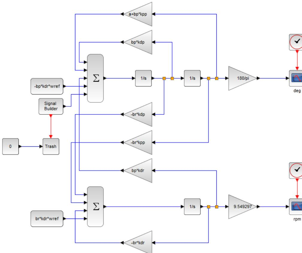
Fig. 3. Subsystem for working out a solution to system ODEs (6) (wheel angular velocity)
