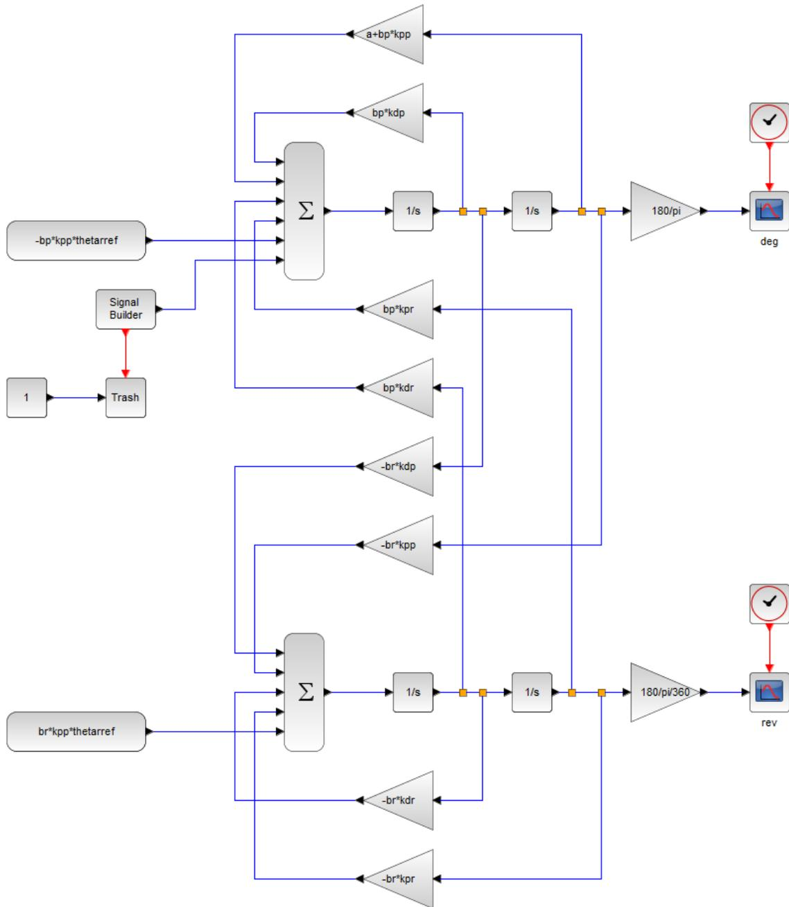
Fig. 4. Subsystem for working out a solution to system ODEs (8) (wheel angle)
